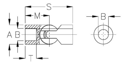
$\begin{array}{lll} A & = 80 \\ B \ H7 & = 50 \\ M & = 115.0 \\ Max \ torque \ (Nm) = 930 \\ s & = 230 \\ T & = 58 \end{array}$
